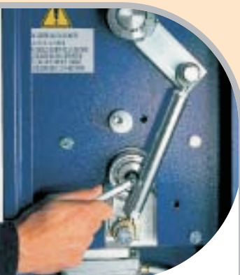
Simple internal unlocking system.
