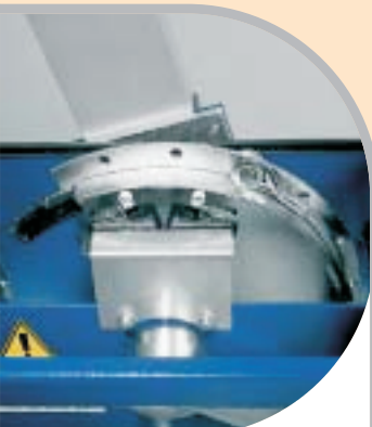
Built-in limit-switch on 230V ac models.
