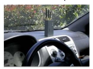
The unit must be vertical with antennas pointing "up" and the unit must be able to "see" the probable locations of the cell phones to be jammed. The unit's effect goes right through plastic panels, or glass or plexiglass windows. A good place in a car is on the dash board or on the rear window shelf, attached with Velcro®.
